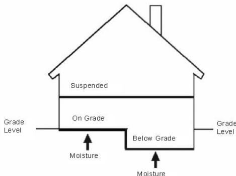
**Above Grade** – An acceptable above grade floor is a concrete or wood substrate.
