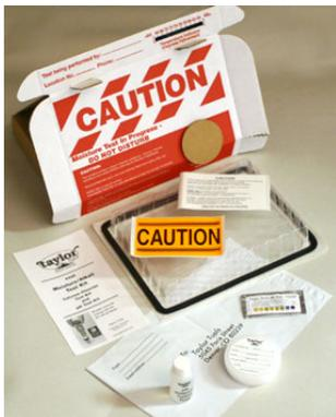
3. Testing for moisture using a Calcium Chloride test kit (**ASTM F 1869 Standard Test Method for Measuring Vapour Emission Rate of Concrete Subfloor Using Anhydrous Calcium Chloride**) will require 3 tests for the first 1,000 sq. ft.
